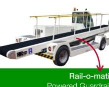
Rail-o-matic Powered Guardrails Remote Control
