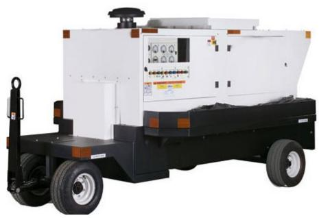
The GPU 4140 ground power unit is a diesel-powered generator that provides regulated 140kVA, 400 Hz, 115/200 VAC, 3-phase power to aircraft. with the 28.5 VDC rectifier option, the unit provides power to aircraft that need 28 VDC at 500A continuous and 2000 A peak. The unit is portable, easy to maintain and durable with uncompromising performance
